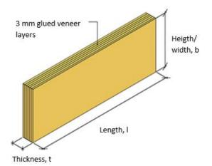
Stora Enso LVL. In S-grade and T-grade all veneers has the fiber direction running parallel to the longitudinal direction. In X-grade the veneers are regularly placed crosswise and parallel to the beam's longitudinal direction
