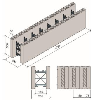
Fig. 5 Thermomur 250X standard block (dimensions in mm)
