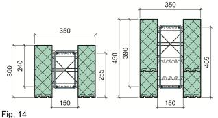
Reinforcement of beams above openings
