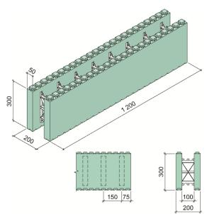
Fig. 4 Thermomur 200 standard block (dimensions in mm)
